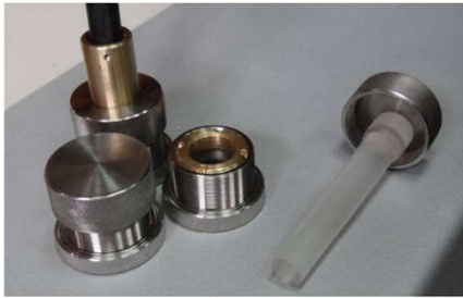
Figure 4. High-voltage connector unit of the PIR-200M consist of 3 sockets.
