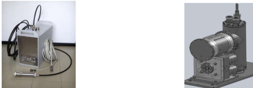
Figure 1. General view of the PIR-200M pulsed X-ray device (left); internal layout (right).
