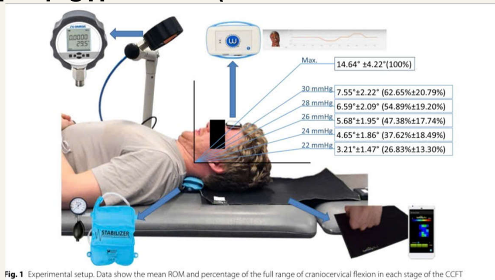
Fig. 1 Experimental setup. Data show the mean ROM and percentage of the full range of craniocervical flexion in each stage of the CCFT
