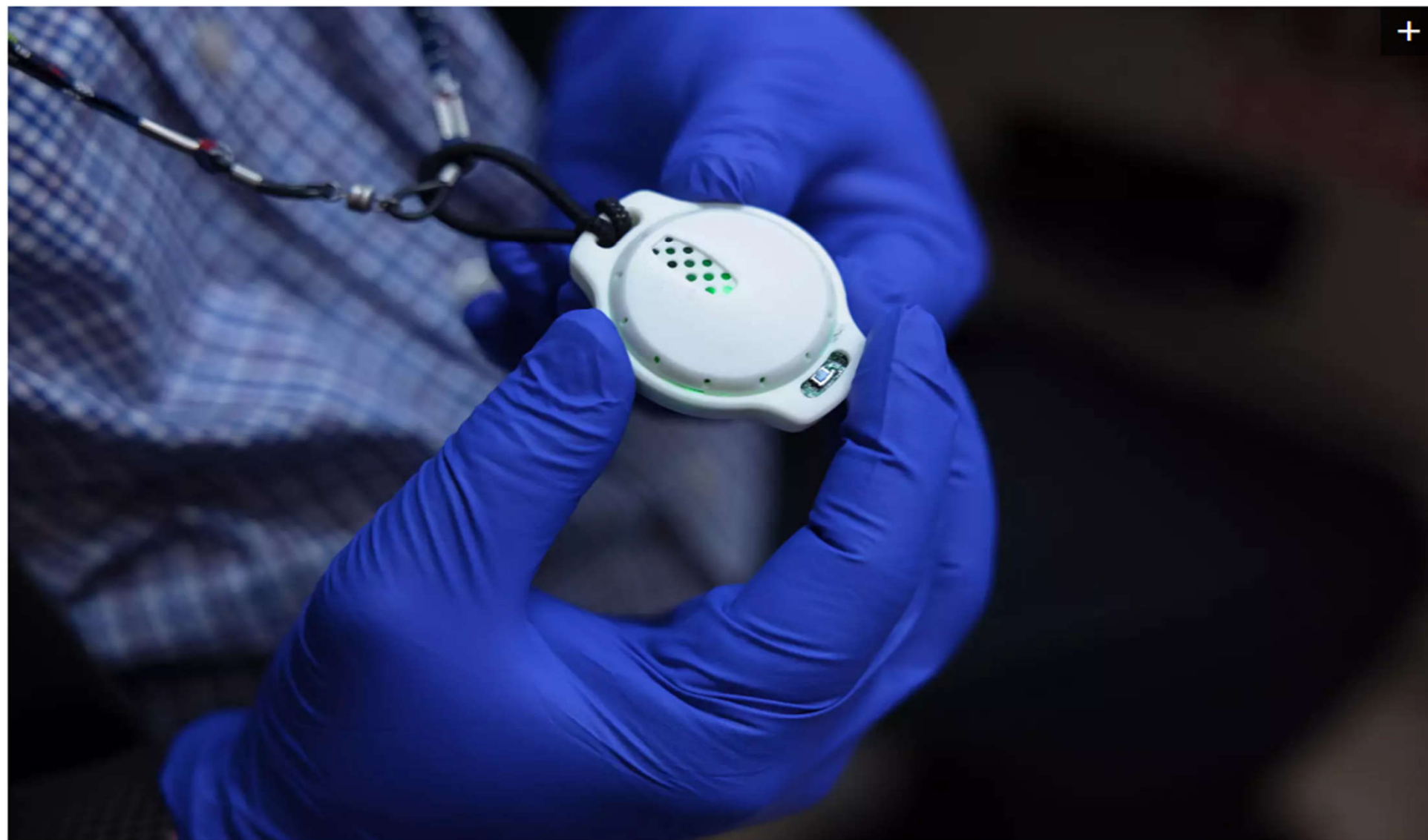
A prototype of isaac by PreEvt, a small lightweight device that can be worn on a lanyard to provide easy and accurate information about blood sugar levels from breath, developed based on research from the Integrated Nanosystems Development Institute at IU Indianapolis. Photo by Liz Kaye, Indiana University
